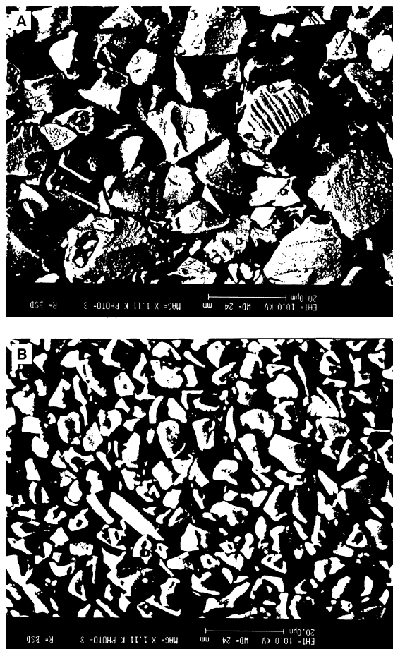
Fig. 1. Micrographic comparison of traditional TLC plates (a), with HPTLC plates (b).
